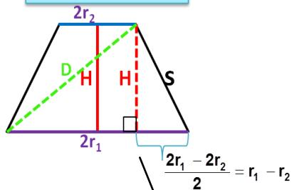
$$P_{\text{оп}} = \frac{2r_1 + 2r_2}{2} H = (r_1 + r_2) H$$
