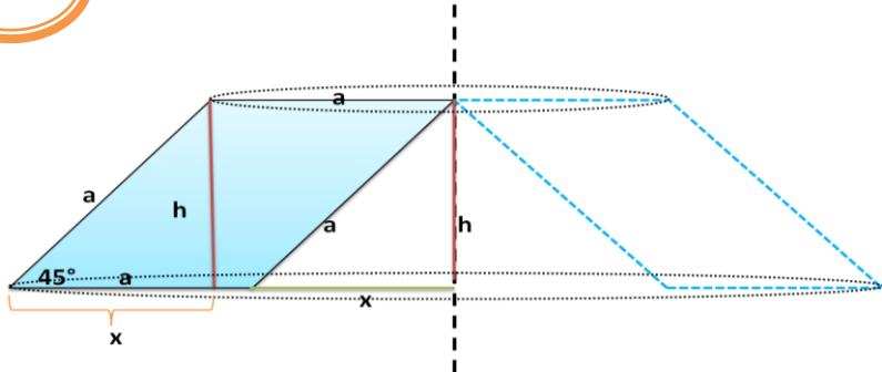
$$\begin{aligned} a &= 3 \\ h^2 + x^2 &= a^2 \\ h = x &\Rightarrow h^2 + h^2 = a^2 \\ 2h^2 &= 9 \Rightarrow h = \frac{3}{\sqrt{2}} = x \end{aligned}$$
